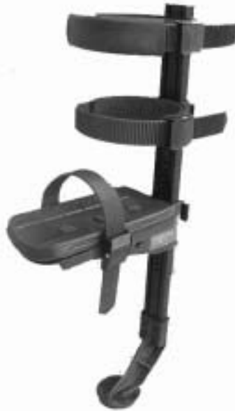
Figure 1: Pictorial representation of the hands-free crutch (HFC). The HFC consists of four components: a vertical telescopic beam allowing for varying user heights; a tibial tray attached to the vertical beam by a pin; two straps above the knee with quick release buckles to secure the thigh to the beam; and one strap below the knee with quick release buckles to secure the lower leg to the tibial tray.
